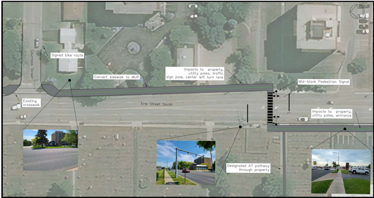
Figure 8-12 MUP with AT Facilities Connection to MUP along East and West Side of Erie Street
