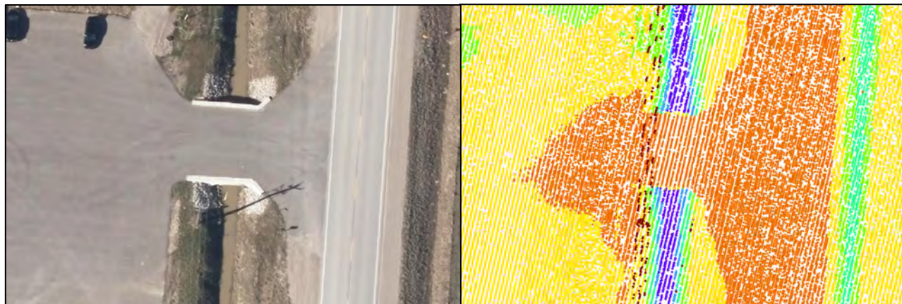
Figure D1 – Aerial and Lidar Point Cloud Plan View of Box Culvert
